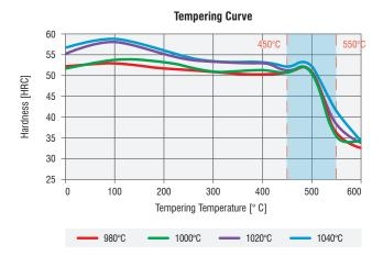
Tempering curve of KeyLos® 2085 samples austenitised at different temperatures between 980°C and 1.040 °C.
