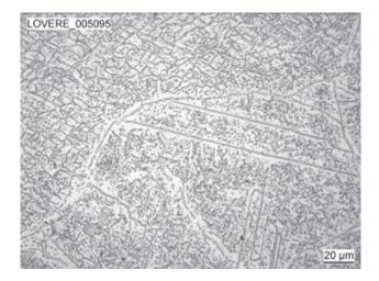
ESKYLOS 2085 in hardening condition: Tempered Martensite with dispersed Carbides
